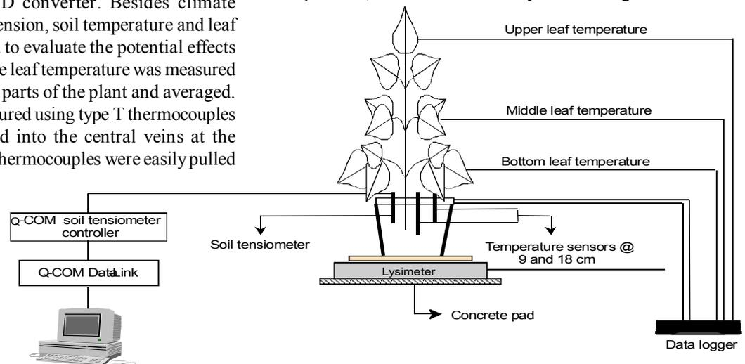
Fig. 1. Schematic drawing of instrumental setup for Red Maple
