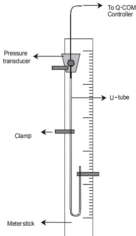
**Fig. 2. Calibration of the tensiometer by aid of Q-COM controller**
